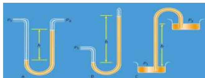
Figure 19. Schematic representations of: (A) differential manometer, (B) Torricelli barometer and (C) siphon
