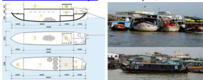
Figure 78. House-boat in the Mekong River Delta - main functional areas: (1) storage, (2) bedroom and kitchen, (3) technical room, (4) water tank, (5) toilet, (6) front part of the boat, (7) deck, (8) rear area (According to: Vu, T.H.H. & Viet Duong, V., 2016)
