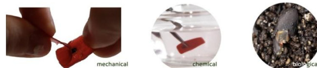
Fig. 4 End-of-Life Strategies for Biobased Nail Interfaces: The mechanical method involves separating the layers and pulling out the electronics. The chemical method dissolves the substrate biomaterial in water or vinegar. The biological method decomposes the biomaterial substrate in a soil mixture containing micro-organisms. These methods can be combined for more effective degradation.
