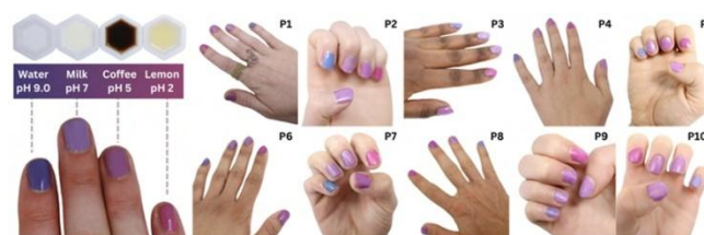
Fig.1 Testing the pH of four beverages with Nail pHolish app, and results on participants' fingernails.
