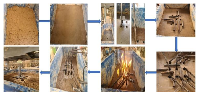
Plate (4): Stages of test procedure of soil improvement by heating for load test
