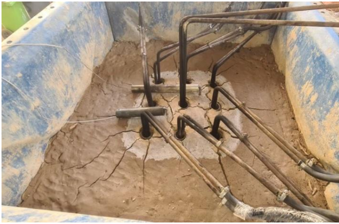
Plate (5): The enhancement area by the heating technique of the 3D model
