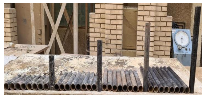
Plate (2): Case tube of the borehole
