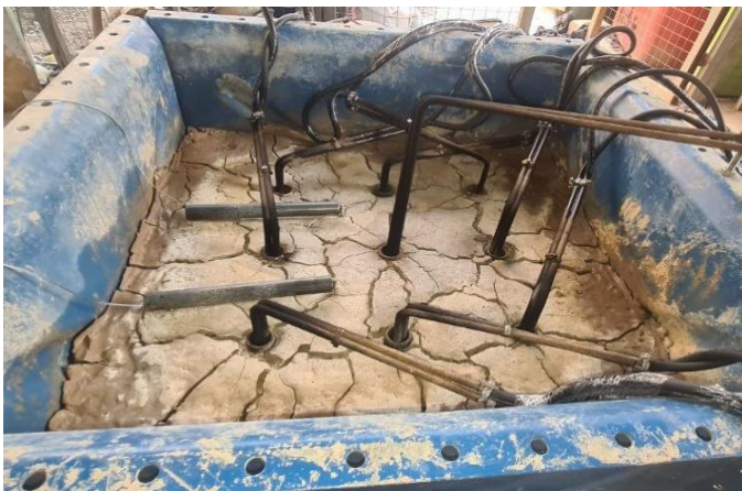
Plate (6): The enhancement area by the heating technique of the 5D model
