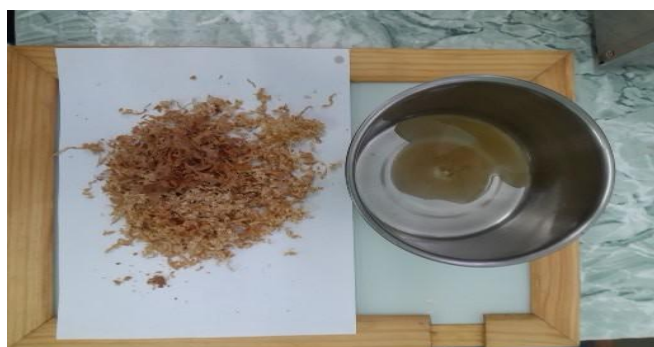
Fig. 3. Press cake and oil recovered from the kernels of plum stones
