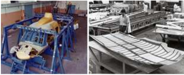
Figure 115. Left: S-75 in final assembly. Right: The lower skin of an S-75 helicopter
