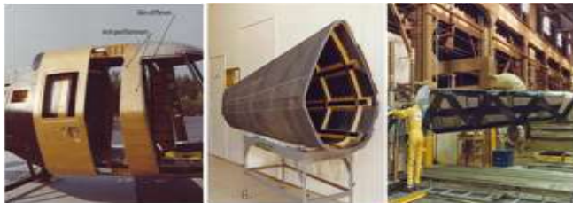
Figure 117. Left: Pre-hung cargo door system. Middle: Left: One-piece tail tip structure. Right: Filament winding of the skin on the tail
