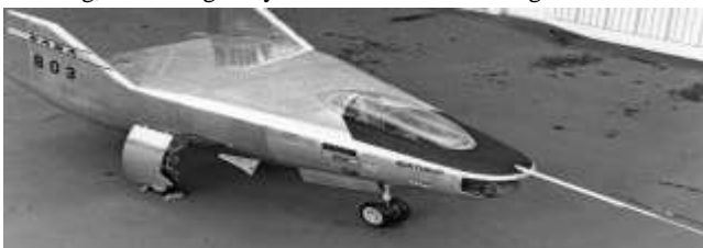
Figure 73. NASA's M2-F2 Lift Body Research Vehicle, 1965 This experimental craft was designed to demonstrate how lift body spacecraft would perform in Earth's atmosphere between reentry and landing.
