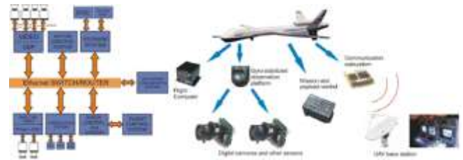
Figure 126. Basic parts of an unmanned aerial vehicle
