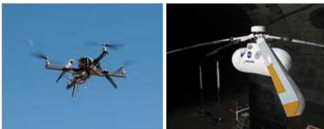
Figure 22. Left: NASA uses a four-rotor model helicopter to test how a four-rotor vehicle can be remotely piloted. Right: NASA tested this rotor design in a wind tunnel to investigate ways to make helicopters quieter.
