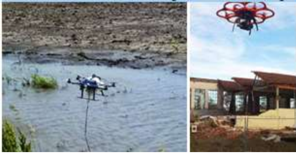
Figure 128. Left: UAV-based camera in river (lake) monitoring. Right: UAV-based camera for structural damage assessment
