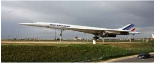
Figure 72. Concorde - a supersonic passenger transport that first flew in 1969 and entered commercial service in 1976. The British Aircraft Corporation and Aérospatiale of France built the aircraft, which was powered by four Rolls-Royce/SNECMA engines.
