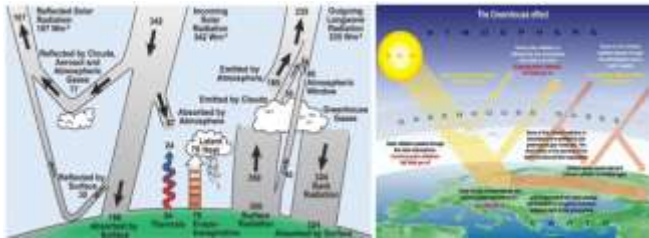
Figure 9. Left: mean annual balance of radiation and heat of the Earth. Right: The Greenhouse effect
