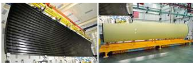
Figure 93. A350 fuselage side panel. Source: Spirit
