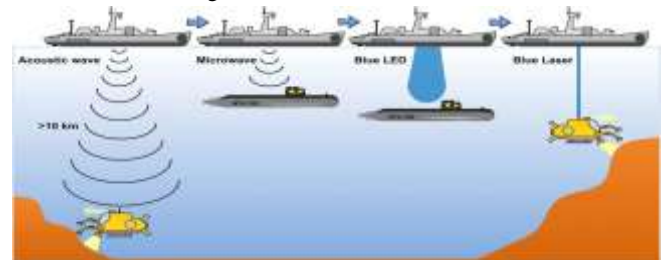
Figure 17. Scheme of the underwater communication system. Scheme of underwater communications based on acoustic waves, microwaves, blue LED and blue LD
